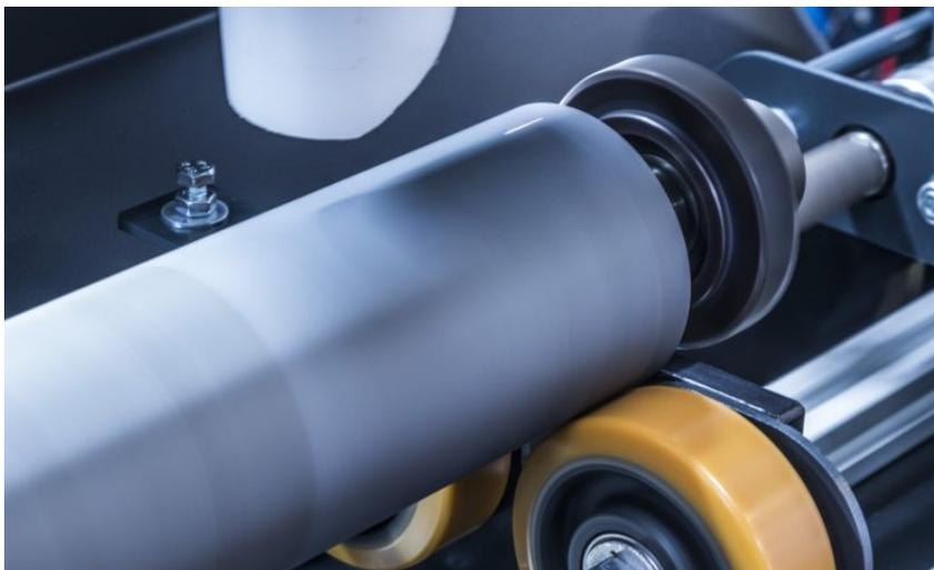
An anilox roller being cleaned with a laser
